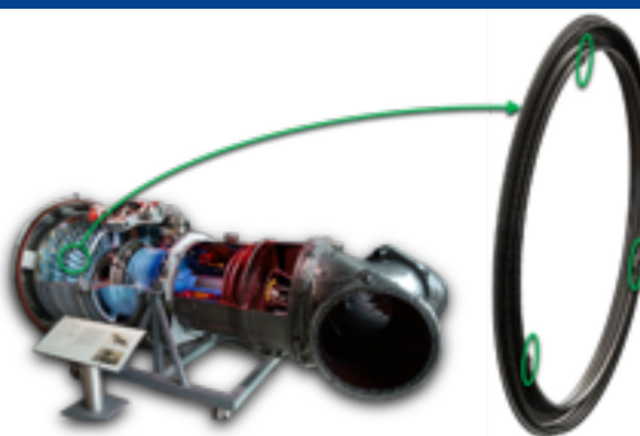
Figure 4: Cutaway view of F402 engine, with CAD representation of the LPC 2nd stage rear seal ring, designating its location within the engine, along with the sites (green ellipses) of typical fretting wear
